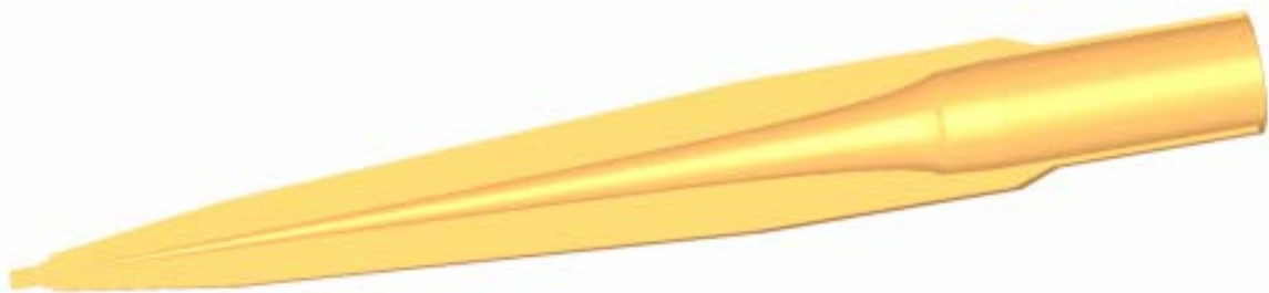
Fig.2a Mathematical optimisation of the n-converter shape
